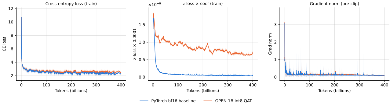
Figure 7 Training curves for OPEN-1B (int8 QAT) versus the bf16 PyTorch baseline. Lines show the rolling mean and shaded bands show \pm 1 standard deviation. Left: train cross-entropy loss. Middle: train z-loss scaled by its coefficient ( 1e-4 ). Right: gradient norm pre-clip.
